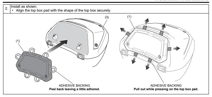
3. Applying adequate pressure of 5 kgf (50 N) to the attached top box pad, and then release the adequate pressure and leave the top box pad for 10 minutes to stabilize the fitting of the adhesive surface.
